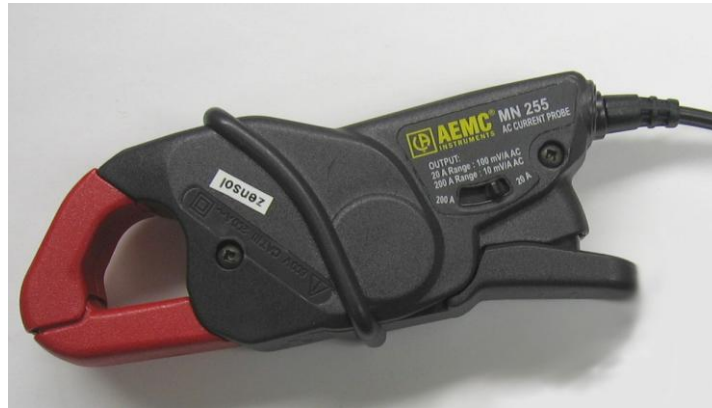
AC Current Clamp (Voltage sensitivity: 100 mV/A AC)
