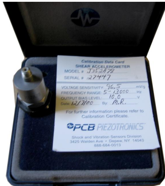
PCB Accelerometer (Voltage sensitivity: around 100mV/G)
