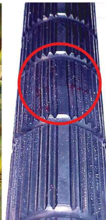
Transmission shaft distortion
