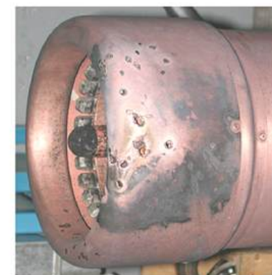
Arc pitting on fixed contacts
